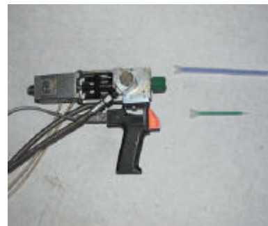
Graphic 5 : Mobile mixing head with static mixing tube.
