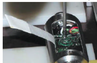
Graphic 4 : Sealing of a sensor with high-temperature gel ISO-PUR A 776.
