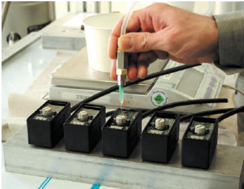
Graphic 3 : Coating with circuit board lacquer ISO-RC 4000 by means of a one-component dispenser.
