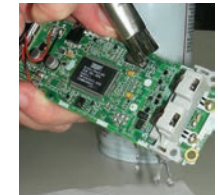
Rinsing the board perfects the cleaning.
