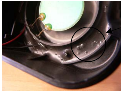
Figure 9. Definite appearance of bubbles in the whole casting
