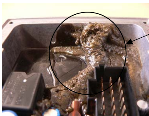
Figure 12: Large areas of not sufficiently mixed cast resin
