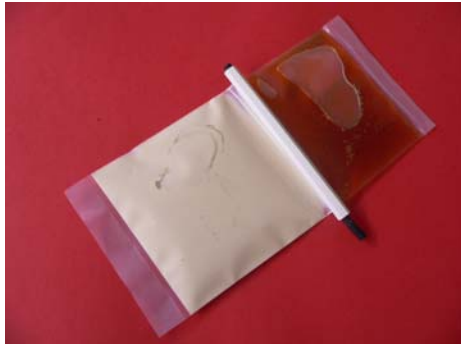
figure 4: ISO – PUR K 711 S 80 cast resin with good thermal conductivity
