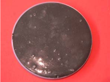
figure 2: Air bubbles were mixed in this sample
